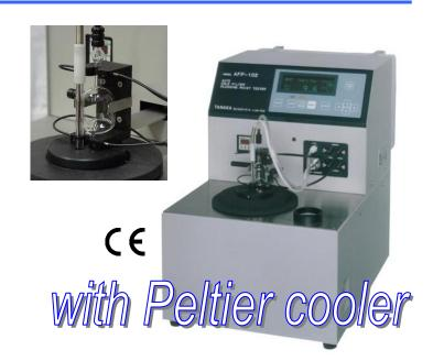
The model AFP-102 automatically executes the Cold Filter Plugging Point (CFPP) test method prescribed in IP309, ASTM D6371 and JIS K2288. After developing its predecessor models, this third generation model has been developed by applying Tanaka's latest technologies and the various know-hows. "Ease of operation" has been further improved on this model.
