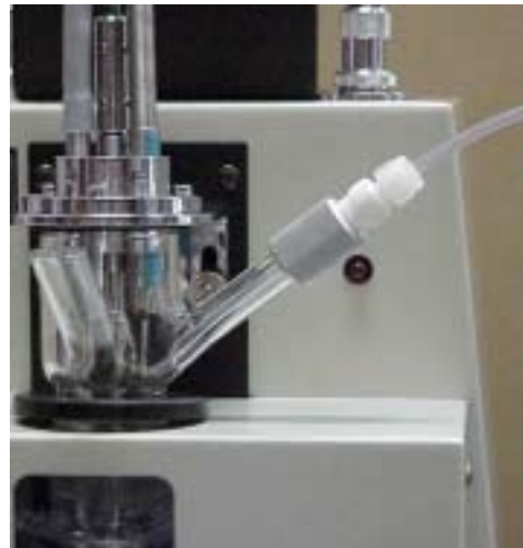
TFE tubing connected to measuring cell for direct connection to bottle-top dispenser for a safer aniline handling. TFE tubing and fitting not provided with AAP-5.
